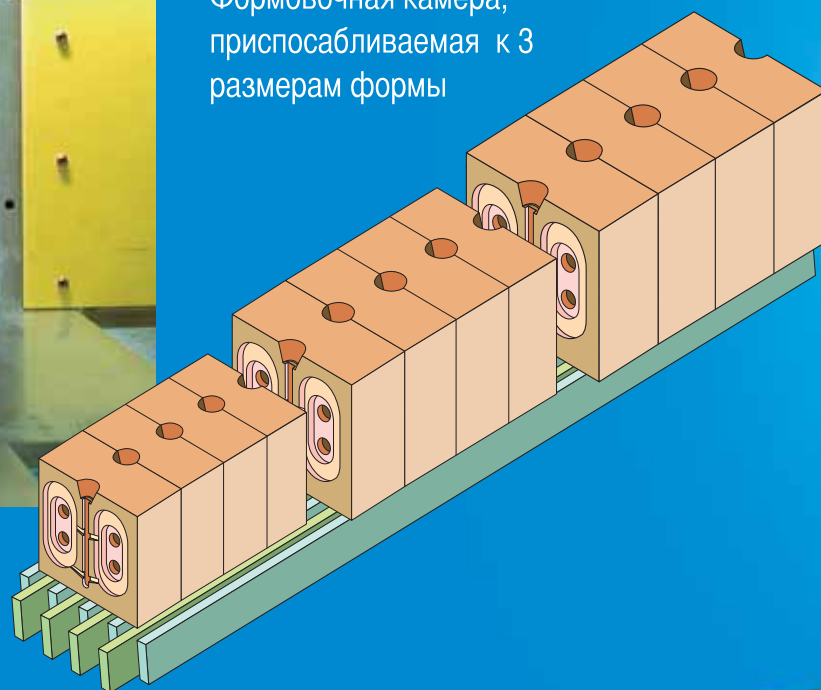
Moulding chamber adaptable to three mould sizes
